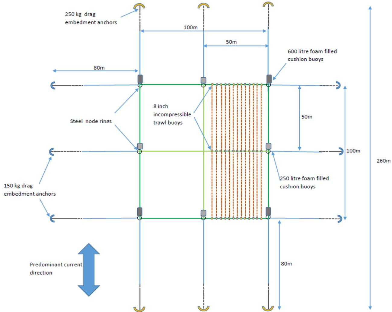
100x100m grid with the capacity for 2.4 kilometre of line. We would like to expand our site by deploying a second larger grid whilst increasing stocking densities and developing surface cultivation systems
